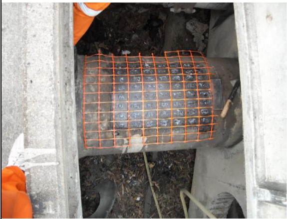
C: Pipe Wall Thickness Measurement in progress.
