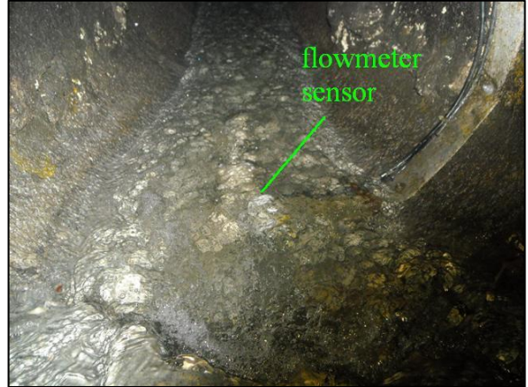
Figure 3.10 Flowmeter in Deeper Flow
