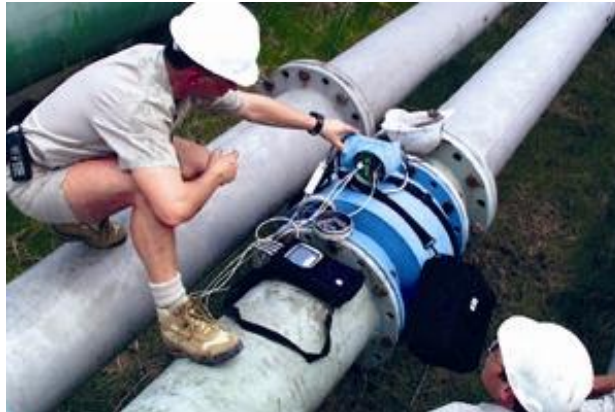
Figure 2.1 An Inline Ultrasonic Flowmeter (Adapted from http://www.controlengurope.com/ )
