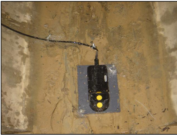
Figure 3.11 Sonic Flowmeter in Silt
