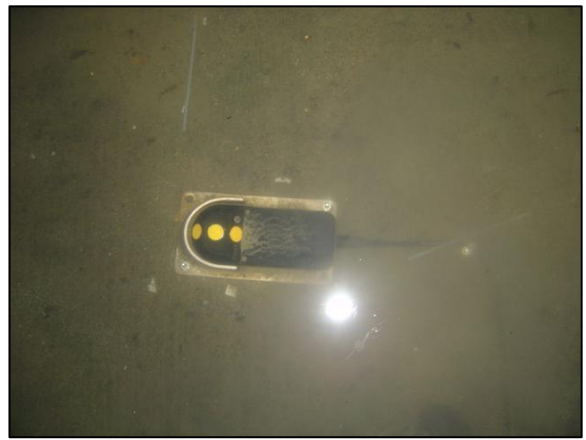
Figure 3.12 Sonic Flowmeter in Shallow Flow
