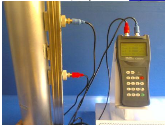
Figure 2.2 A Clamped-on Handheld Ultrasonic Flowmeter (Adapted from http://theultrasonicflowmeters.com/ )
