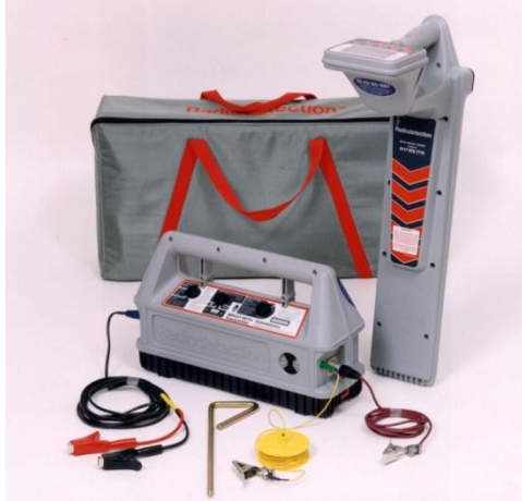
A: A locating set for direct connection method.
