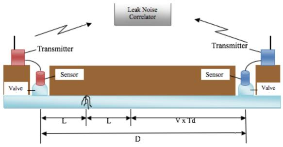
Fig. 4.1.1.2 Sample set up of LNC Survey.
