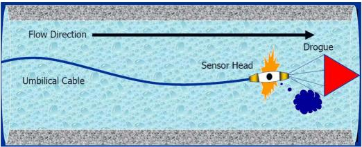
Figure 4.1.5.2 The drogue used to propel the Sahara sensor through the pipeline.
