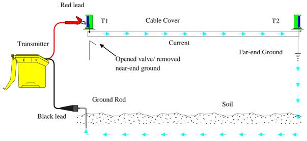
Fig. 4.1 Direct connection method
