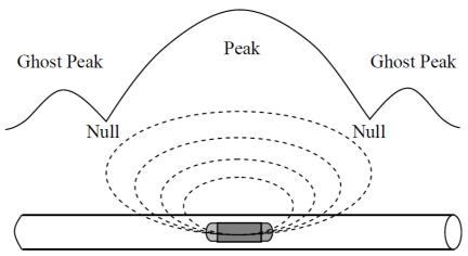
Fig. 4.4 Pattern of the signal response when detecting a sonde
