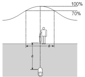
Fig. 4.6 Measuring depth by 70% method
