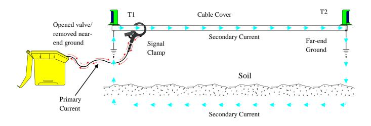
Fig. 4.2 Signal clamping
